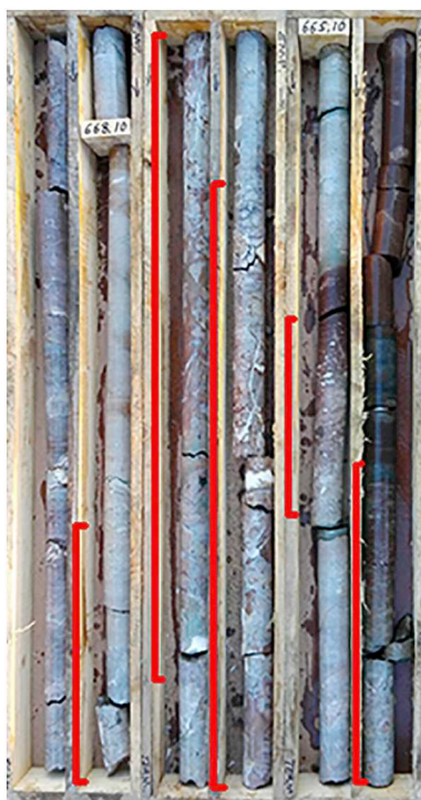
Fig. 5. Partial section (664.3 m to 668.9 m) of the lithologic log from Villabona Mine (Courtesy of the Minersa Group). This part of the section represents the karst on the top of the Sotres Formation. Lateral equivalents to the karst are shown in Peña Careses, east Oviedo (Fig. 6B), and in the Carmona section (Fig. 9i). Vertical (red) lines mark some levels of breccias originated by dissolution (karstification). Part of the karst in the lithologic log is mineralized with fluorite, being this mineral the main objective of the exploration in the mine. Total thickness of the Sotres Formation in the lithologic log from Villabona Mine reaches 7.10 m. (For interpretation of the references to colour in this figure legend, the reader is referred to the web version of this article.)
