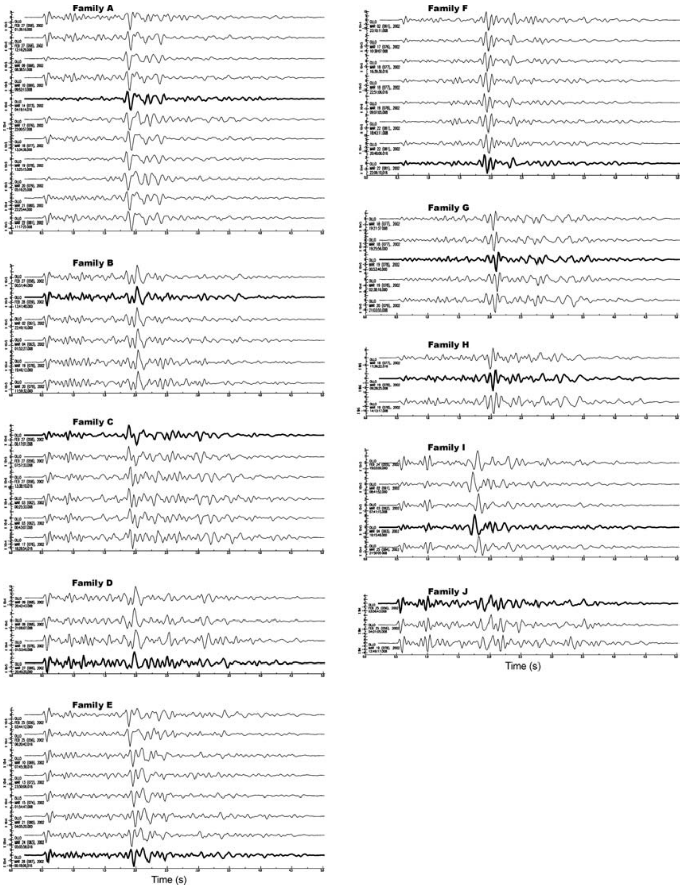
Figure 9. Vertical component seismograms, 3–15 Hz bandpass filtered, recorded at OLL station, of the ten families obtained by correlation analysis. Bold traces are the master events used to cluster event location.
